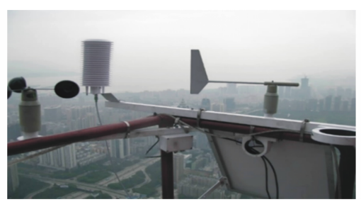
图 4 气象站安装 Fig. 4 Installation of Meteorological Station
