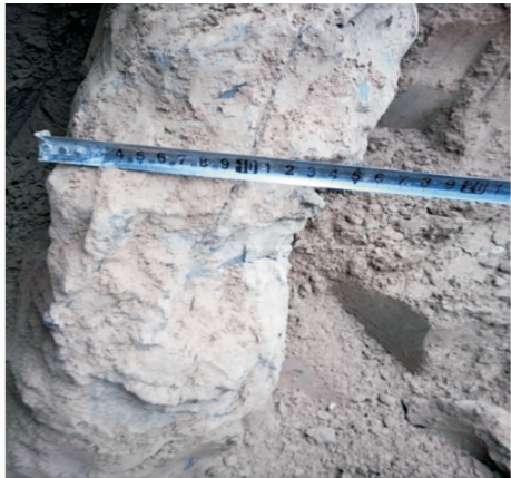
图 3 固结水泥柱扩粗图 Fig. 3 Consolidated Cement Column Expanding Figure
