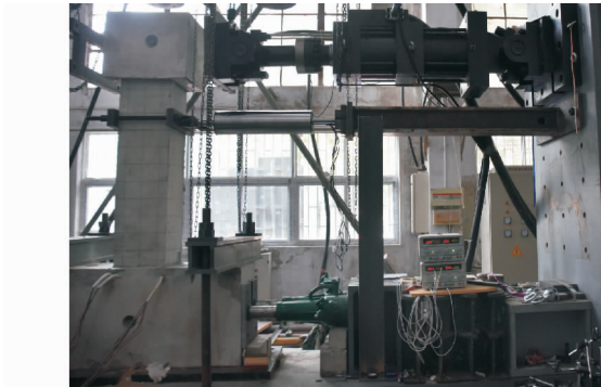
图 8 阻尼器与柱体连接图 Fig. 8 Photo of Connection Between MRD and Column
