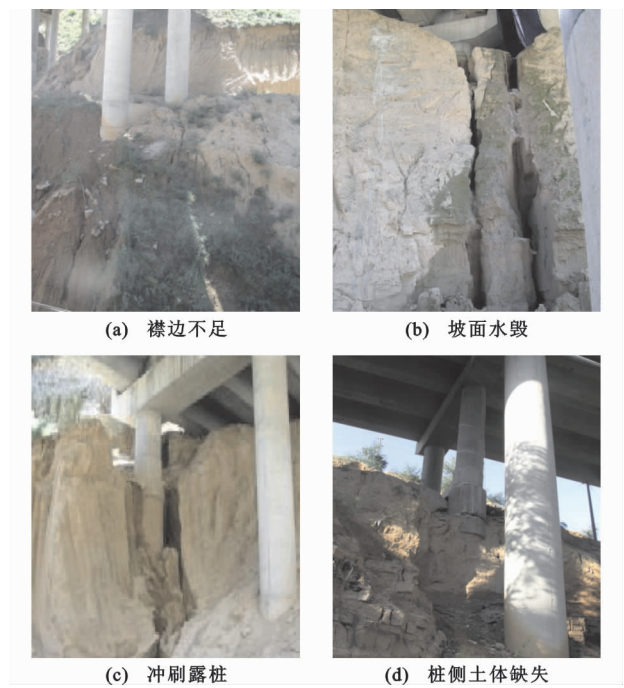
图 1 桩基水毁病害 Fig. 1 Water Damage of Pile Foundation
