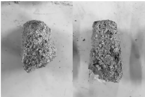
图 2 注浆后典型试样 Fig.2 Typical Samples After Grouting
