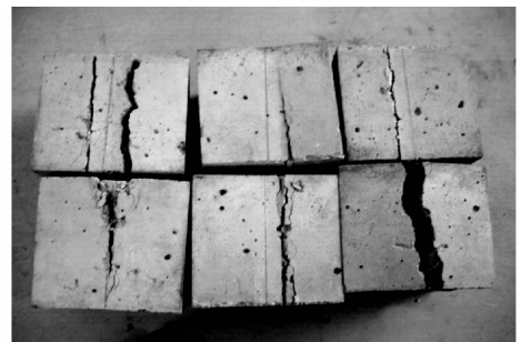
(a) 劈裂破坏
