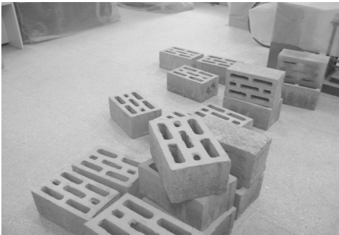
图 1 三排孔再生混凝土砌块 Fig. 1 Recycled Concrete Block with Three-rows Holes
