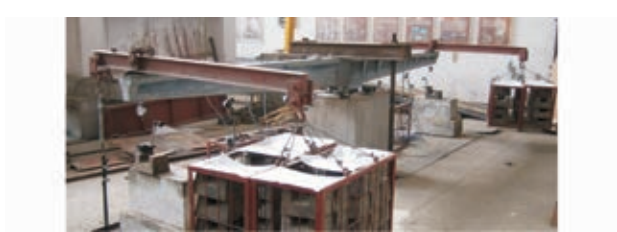
图 32 双悬臂 UHPC 工字梁徐变试验 Fig. 32 Creep Tests on UHPC I-shaped Beam with Double Cantilevers
