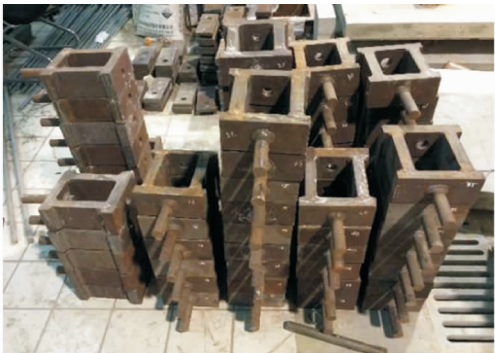
图 4 抗拉试验辅助装置照片 Fig.4 Photo of Auxiliary Device in Tensile Test
