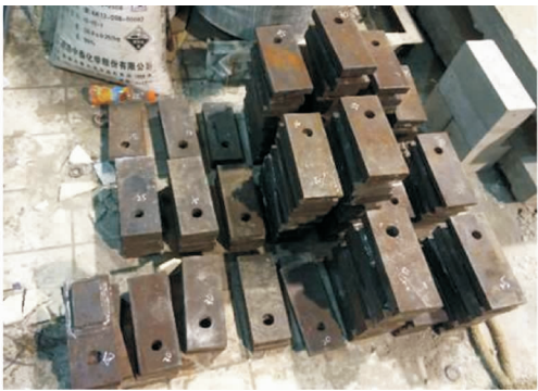
图 6 抗剪试验辅助装置照片 Fig.6 Photo of Auxiliary Device in Shear Test
