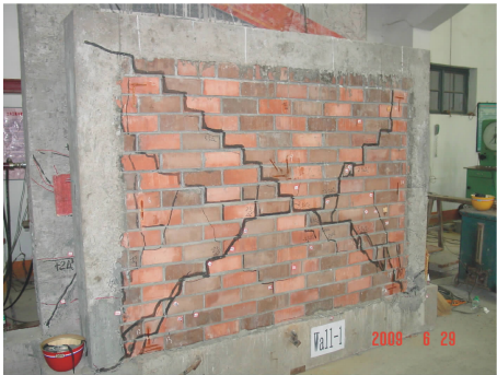
图 8 试件破坏形态 Fig. 8 Failure Form of Specimen
