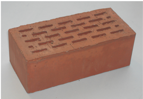
图 2 用污泥制作的陶瓷清水砖 Fig. 2 Ceramic Bricks Produced by Sludge
