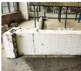
(c) T形梁裂缝破坏情况
