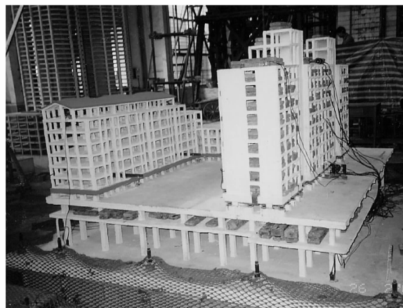
Fig. 10 Shaking Table Tests for Structural Model of IHBSH
