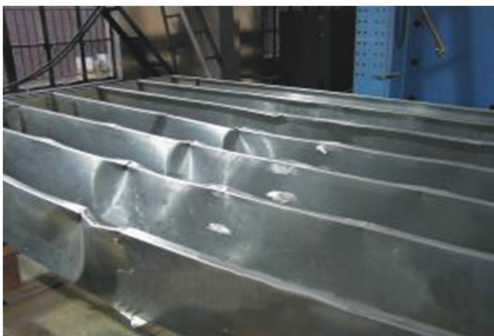
(c) 试件FL-2破坏后的楼盖骨架
