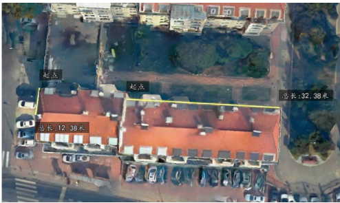
图 2 测量三维建筑模型的平面尺寸 Fig. 2 Measuring plan dimensions of 3D building model
