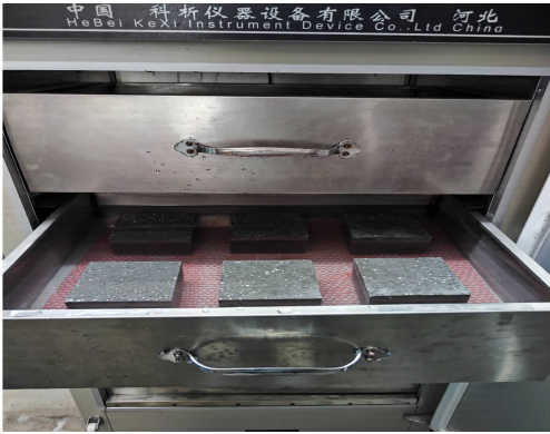
图 3 试件室温浸水养护 Fig. 3 Specimen soaked in water for curing at room temperature
